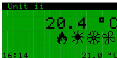
This is the main screen that indicates the current room temperature, the current temperature setpoint, the current time and the unit state. The unit state is depicted by 4 different pictures: gas heating (🔥), heat pump heating (☀️), cooling (❄️), fan (🌀). If the unit is off, the reason is also described on this screen (for example: by scheduler, by terminal or by alarm).
